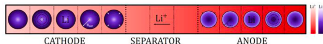
Fig. 4. Schematic representation of the P2D electrochemical model with indicated concentration of Li-ions in electrolyte (red colour) and concentration of Li in particles (purple colour) during a discharge. (For interpretation of the references to colour in this figure legend, the reader is referred to the Web version of this article.)
