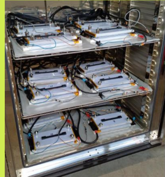
12 li-ion cells tests, Energetic project EDF R&D
