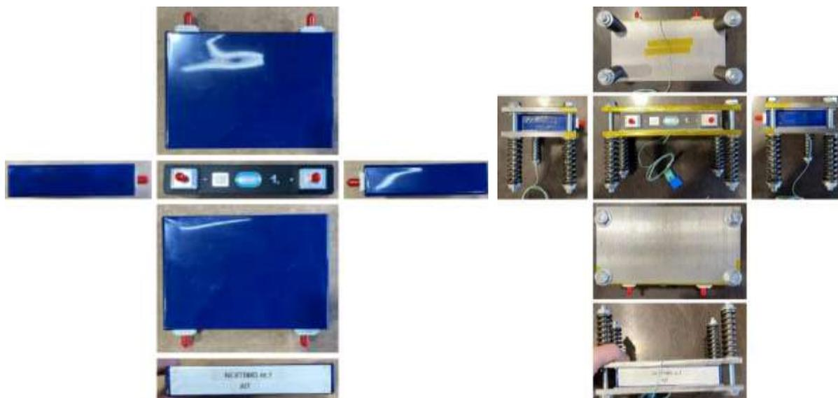
Figure 18: Cell before (left) and after assembly of the clamping plates (right).
