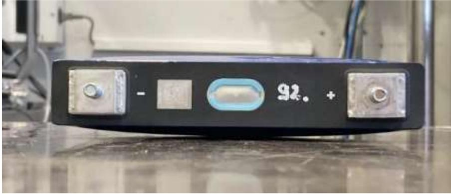
*Figure 30: Optical inspection of the damaged and inflated cell (view on terminal side)*
