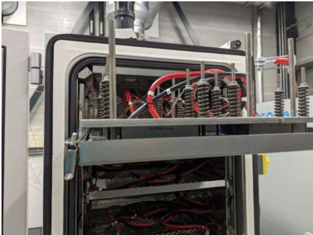
Figure 2: Side view of the tested cells and cell clamps. The cell labels are visible to the careful reader.
