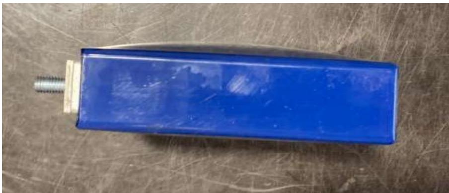
*Figure 31: Optical inspection of the damaged and inflated cell (side view)*
