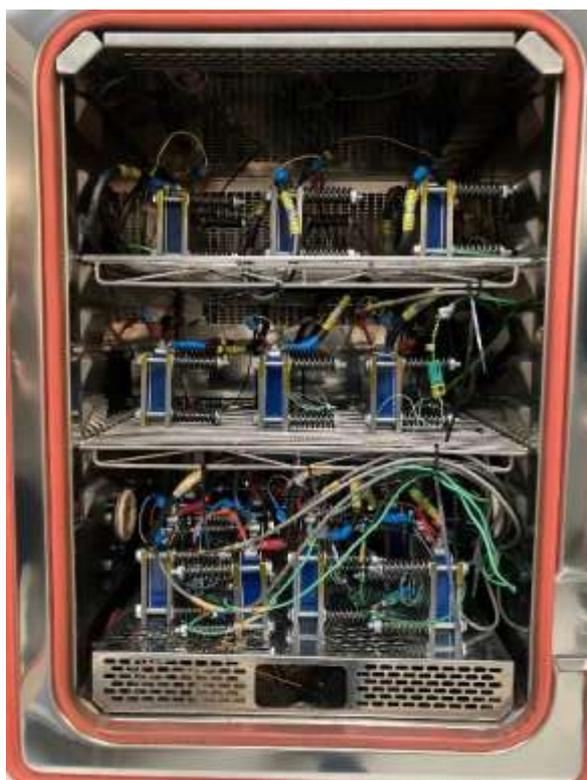
Figure 19: Arrangement of the prepared cells in the climatic chamber
