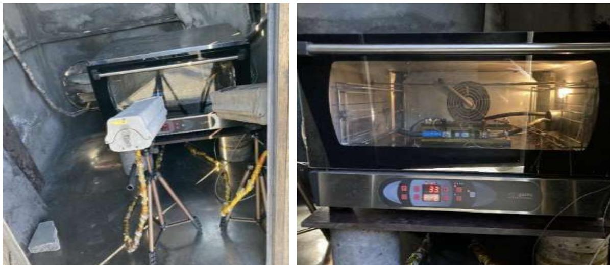
Figure 20: Abuse chamber equipped with cameras (left) and a climatic chamber with arranged cell inside (right).
