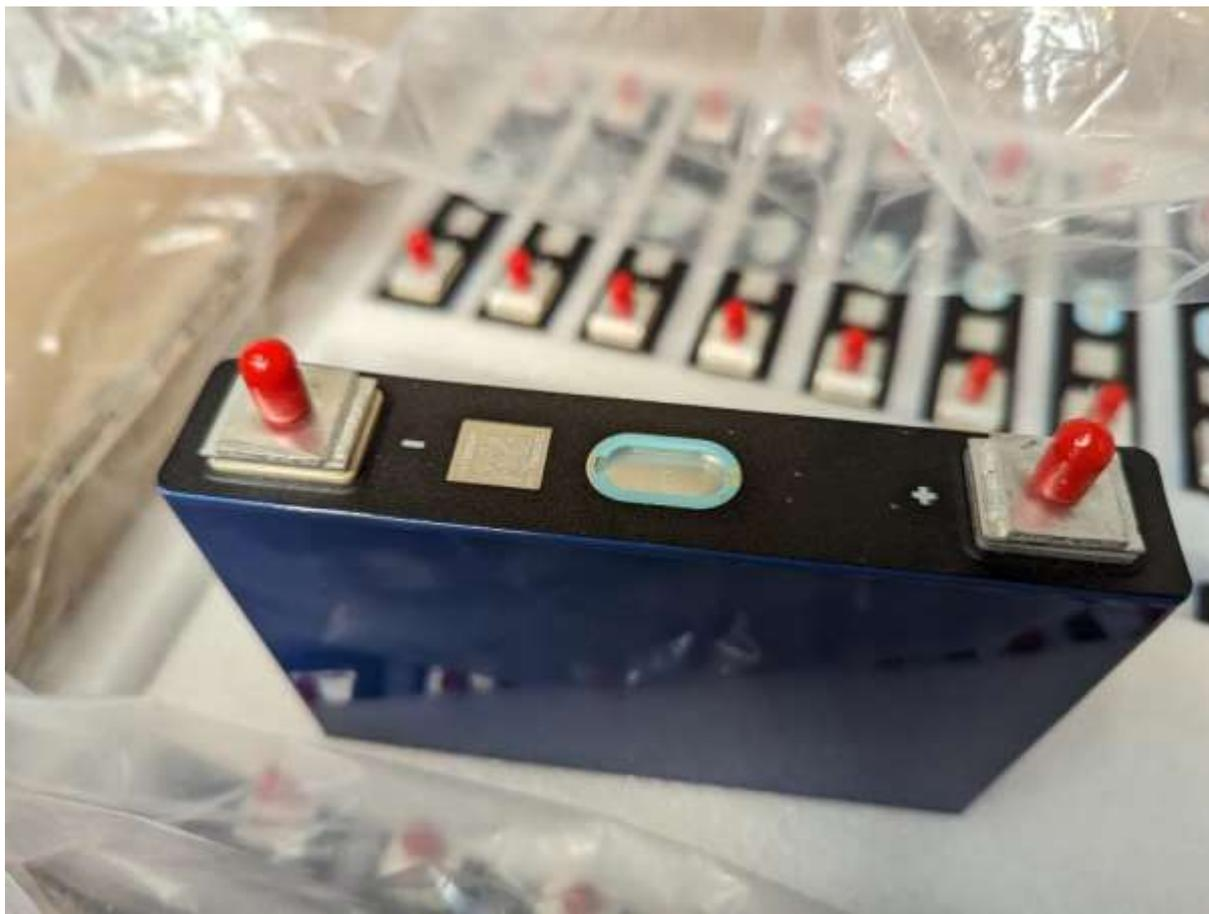
*Figure 1: Example of the acquired 58Ah prismatic cell used in the NEXTBMS project.*
